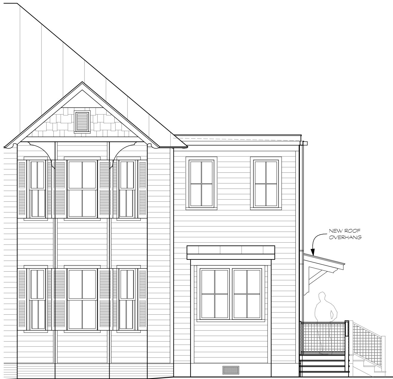
1 HOUSE: PROPOSED SOUTH ELEVATION SCALE: 3/16" = 1'-0" 0 4' 8' 12'
