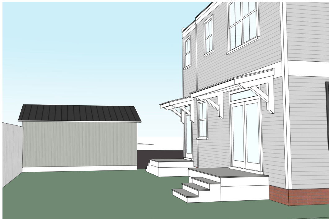
Proposed house roof overhangs, view from North
